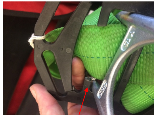
Damage to Plastic clip at "D" ring
